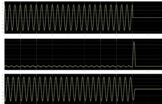
Figure 11: Detection Results of ABG Fault at Point A for A, B and C Phases Respectively for Model 2.
