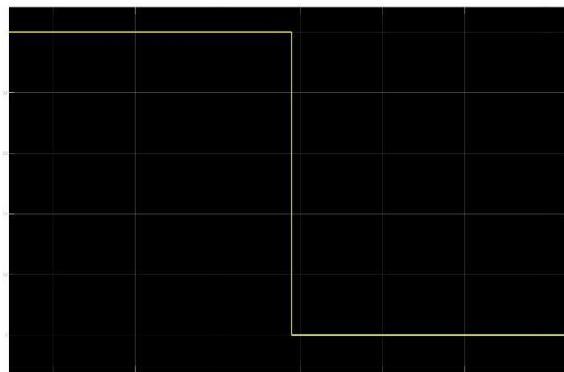
Figure 8: Circuit Breaker Tripping Time Recorded as 6.6 Milliseconds for AB Fault.
